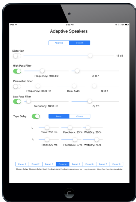
Fig. 4: Mobile application to select desired effects and presets
